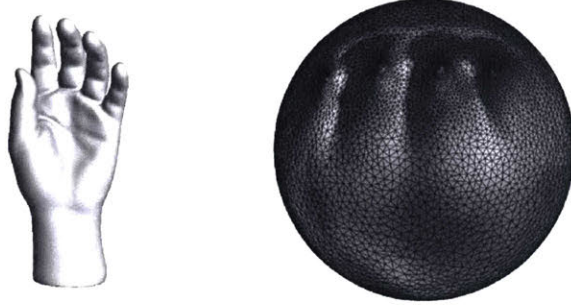
Figure 3-1: A conformal mapping from a complex geometry - a hand - to a sphere. The uniform mesh on the hand is now pinched at certain areas on the sphere, preserving information regarding the structure of the fingers. [1]
